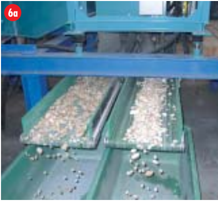
Figs. 6 a-c Sorting of feldspar 15-40 mm, capacity: 30 t/h, reject quantity approx. 40 %
