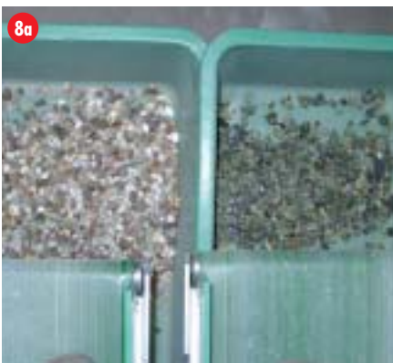
Figs. 8 a-c Sorting of burnt magnesium oxide 10-30 mm, capacity: 25 t/h, reject quantity approx. 30 %
