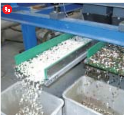
Figs. 9 a-c Sorting of burnt magnesium oxide 8-12 mm, capacity: 20 t/h, reject quantity approx. 40 %
