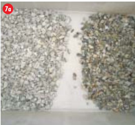
Figs. 7 a-c Sorting of wollastonite 8-20 mm, capacity: 20 t/h, reject quantity approx. 40 %
