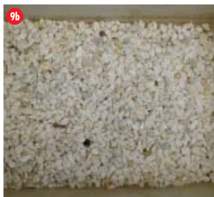
Figs. 9 a-c Sorting of burnt magnesium oxide 8-12 mm, capacity: 20 t/h, reject quantity approx. 40 %
