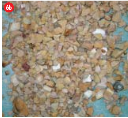
Figs. 6 a-c Sorting of feldspar 15-40 mm, capacity: 30 t/h, reject quantity approx. 40 %
