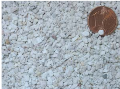
Fired Flint with size range 1,6 - 2,5 mm
